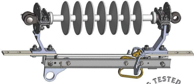
This 15-35kV In-Line Disconnect Switch from Aluma-Form is marine grade (316SS hardware and brackets, with all Aluminium components nickel plated and all hex nuts silicone bronze) and features a 200kV BIL silicone insulator.
