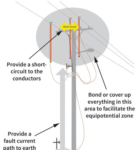
Earthing applied to ensure operation of circuit protection and facilitate creation of equipotential zone at working position.
